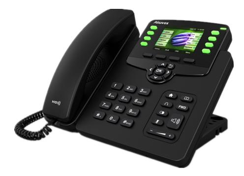
The Akuvox R63G is a featured 3-line IP phone with full duplex hands-free speakerphone. It can be directly connected to an Internet Telephony Service Provider or to an IP PBX.
